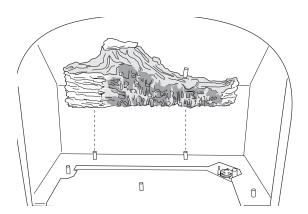
Figure 20. Engage the holes in the underside ot the Rear Log with the two pegs in the burner skirt.
